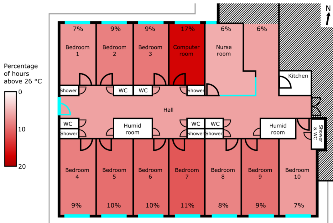
Figure 10. Indoor overheating by room
