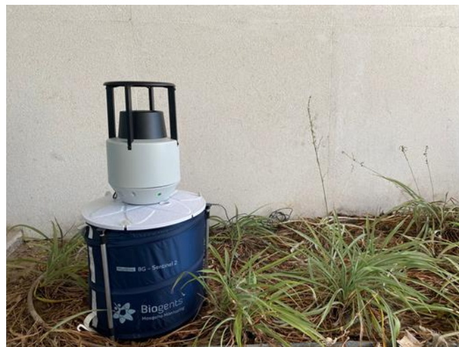
Figure 14: VECTRACK smart-trap set-up: the VECTRACK sensor installed on top of a commercial mosquito trap for professional use, in this case the BG-Sentinel model.
